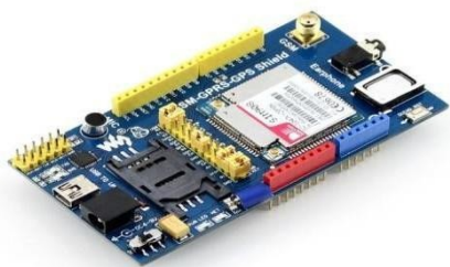
Fig., GS M module to network connection
